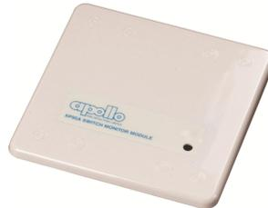
The XP95A Switch Monitor Module is designed to monitor the state of one or more single pole, voltage free contacts connected and to report the status to Apollo compatible analog control equipment.
