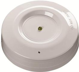
The XP95A Isolator is placed at intervals on the loop and ensures that, in the case of a short circuit, only the section between the isolators will be affected.
